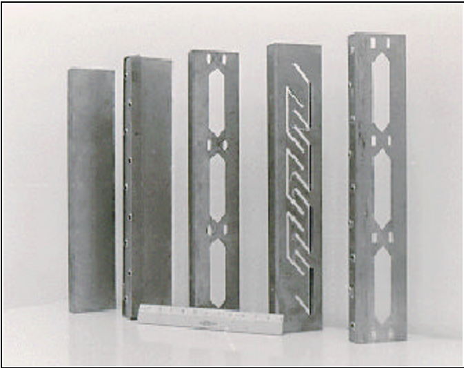
Figure 1: Thermal Steel stud concepts developed and patented by Dofasco.
